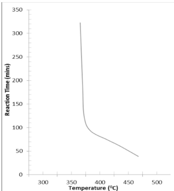
**Fig. 5:** Reaction Time vs Temperature (Pt/Al<sub>2</sub>O<sub>3</sub>).
