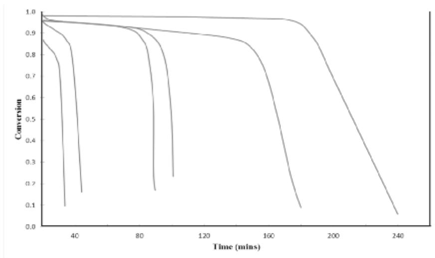
Fig. 2: Conversion vs Time of Reaction (Pt/Al<sub>2</sub>O<sub>3</sub> at 430°C).
