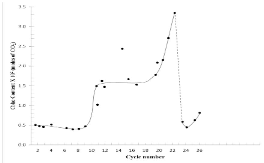
**Fig. 3:** Coke Content vs Cycle Numbers (Pt /Al<sub>2</sub>O<sub>3</sub> at 430°C).
