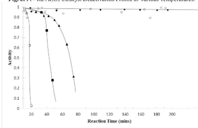
**Fig. 7:** Pt / $\text{Al}_2\text{O}_3$  Catalyst Deactivation Profile at Various Temperatures.
