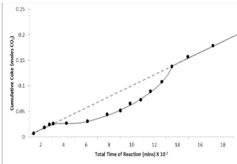
**Fig. 4:** Cumulative Coke Content vs Total Reaction Time (Pt/Al<sub>2</sub>O<sub>3</sub> at 430°C).
