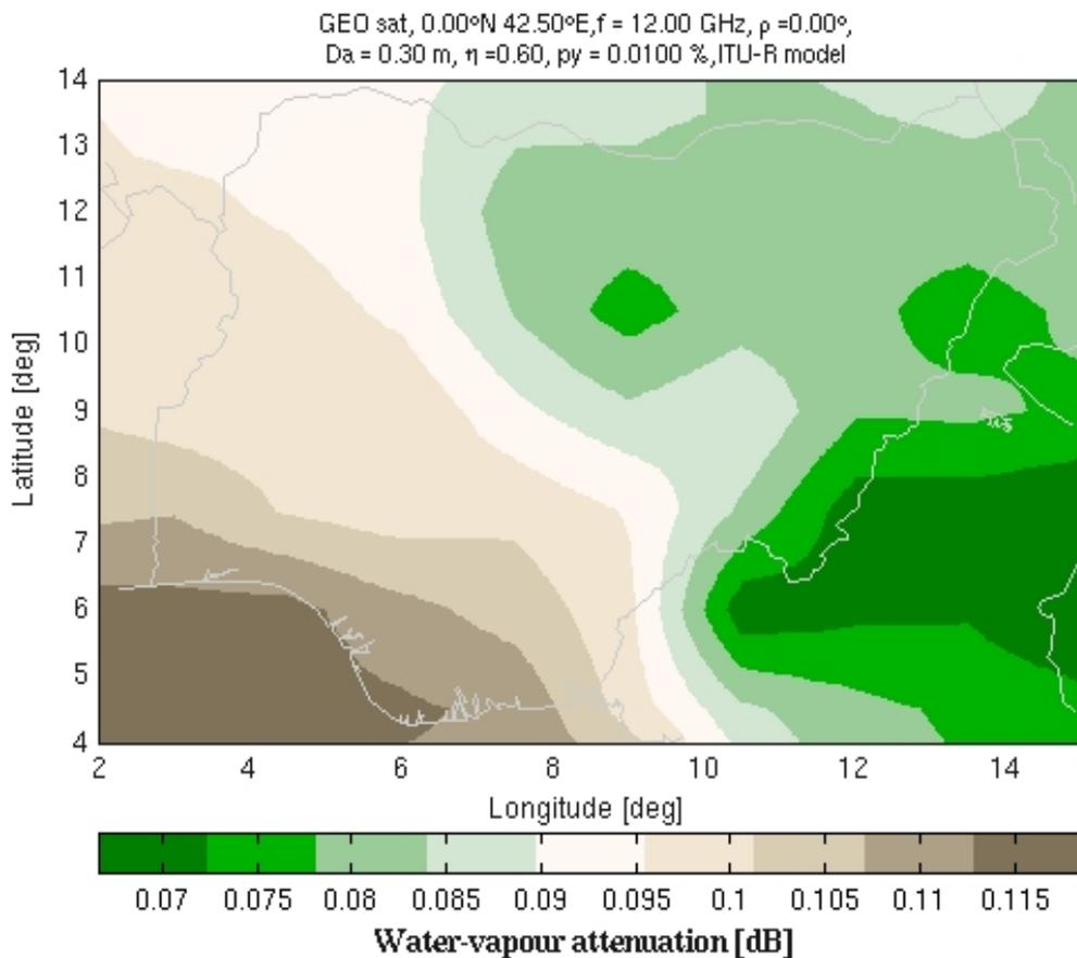
Figure 4. Contour map of water-vapour attenuation for Ku downlink (12 GHz) from NigComsat-1 at 0.01% unavailability
