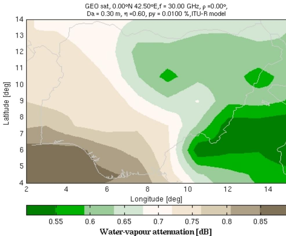
Figure 10. Contour map of water-vapour attenuation for Ka uplink (30 GHz) to NigComsat-1 at 0.01% unavailability.
