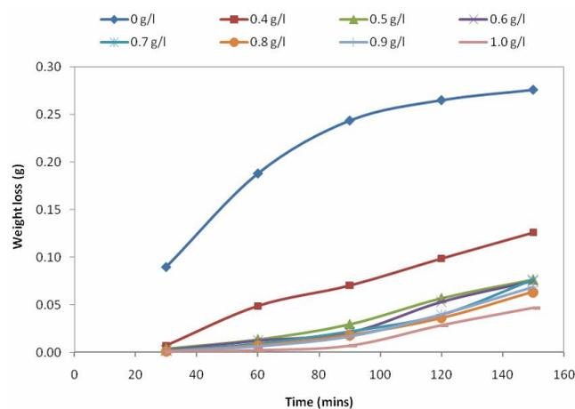
Figure 1 : Variation of weight loss with time by *Vernonia amygdalina* inhibition of aluminium in 0.5M HCl solution.
