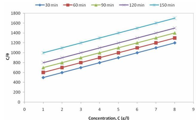
**Figure 3 :** Langmuir adsorption isotherm relationship between  $C$  and  $C/\theta$  for using *Vernonia amygdalina* as inhibitor for aluminium at different exposure time in 0.5M HCl.
