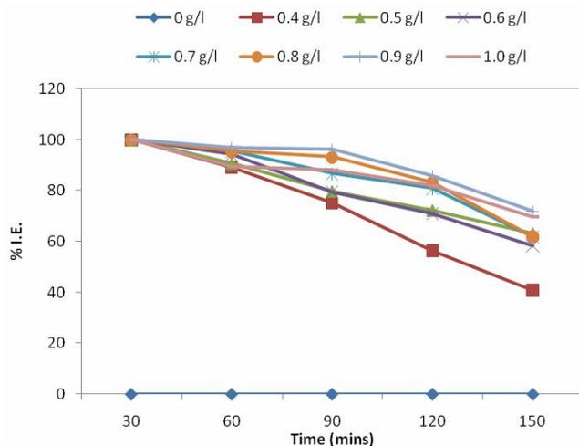
**Figure 2 :** Variation of inhibition efficiency (% I.E) by *Vernonia amygdalina* of aluminium at different exposure time in 0.5M HCl.
