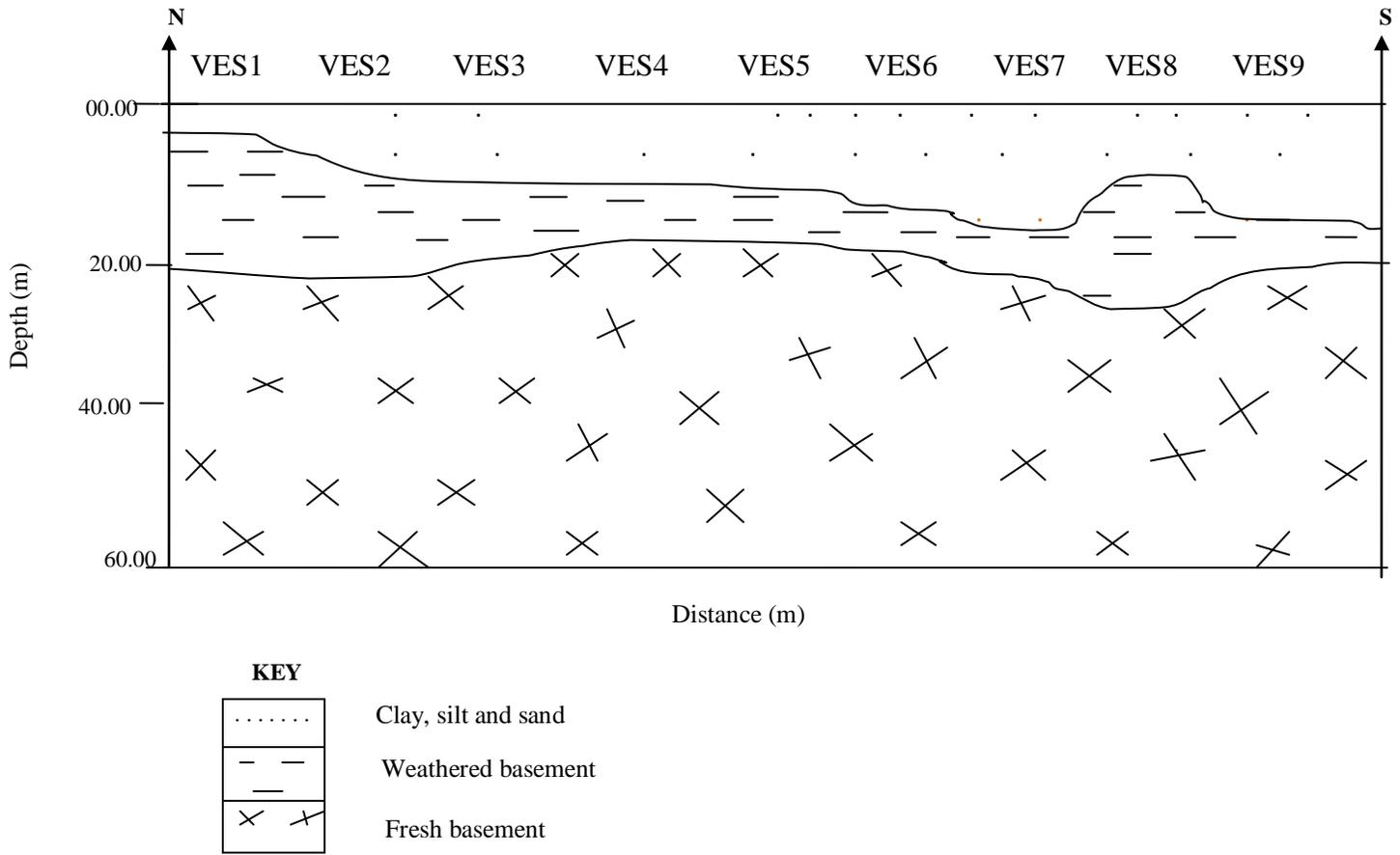
Figure 3.2: Geologic section derived from profile A
