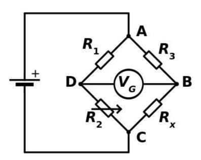
15. If the Wheatstone bridge above is 'balanced' when  $R_1$  = 630  $\,$ ,  $R_2$  = 972  $\,$ , and  $R_3$ = 42.6  $\,$ , what is the value of the unknown resistance?
