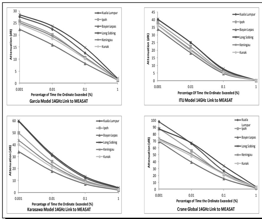
Figure 2b. Rain attenuation (dB) at Ku, (14 GHz) for exceedence probabilities of 0.001-1% of an average year
