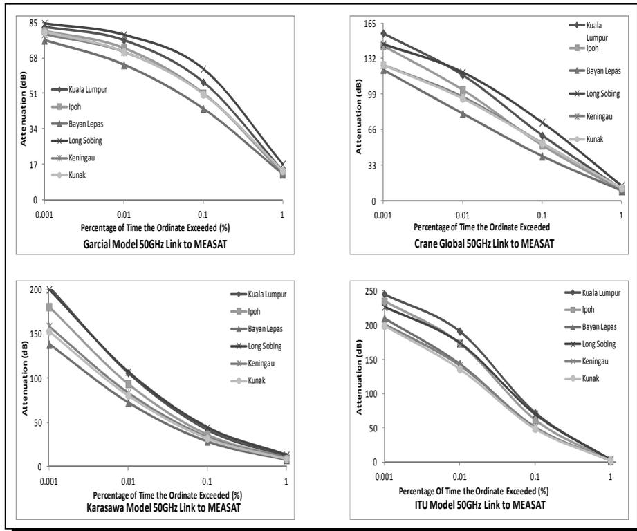
Figure 2f. Rain attenuation (dB) at V (50 GHz) for exceedence probabilities of 0.001-1% of an average year
