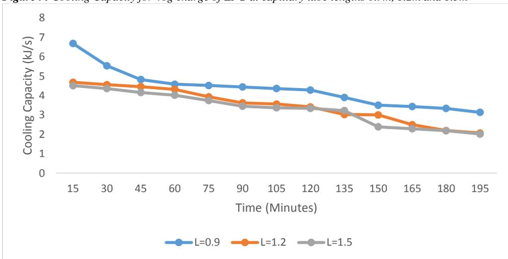
**Figure 10:** Cooling Capacity for 60g charge of LPG at capillary tube lengths 0.9m, 1.2m and 1.5m
