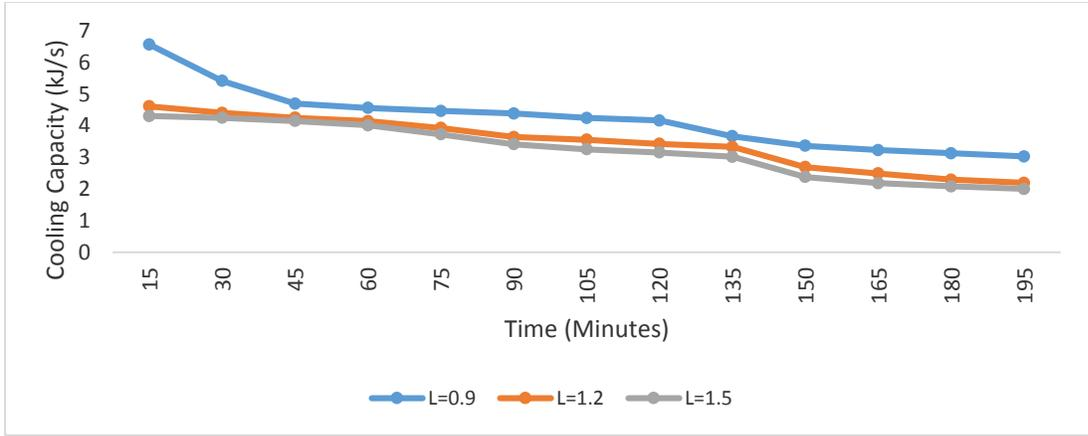
**Figure 8:** Cooling Capacity for 60g charge of R600a at capillary tube lengths 0.9m, 1.2m and 1.5m
