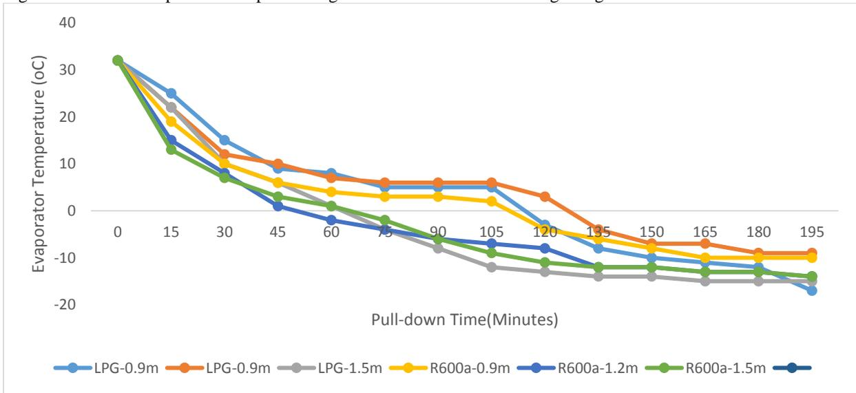
Figure 16: Plot of Evaporator Temperature against Pull - down Time for 60g charge of LPG and R600A
