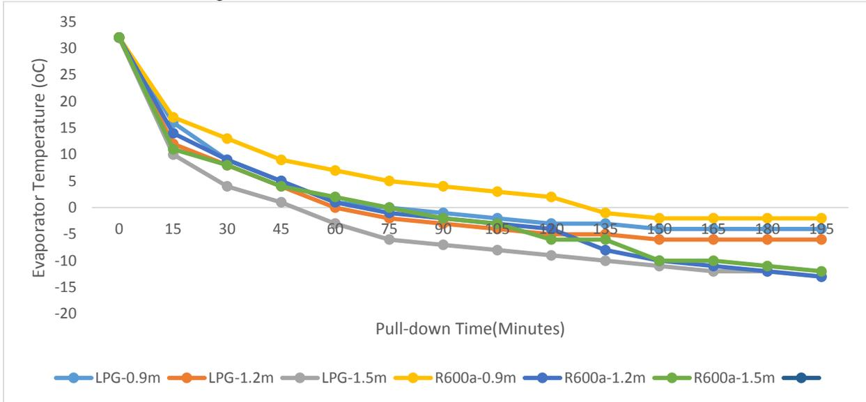
Figure 15: Plot of Evaporator Temperature against Pull- down Time for 40g charge of LPG and R600A
