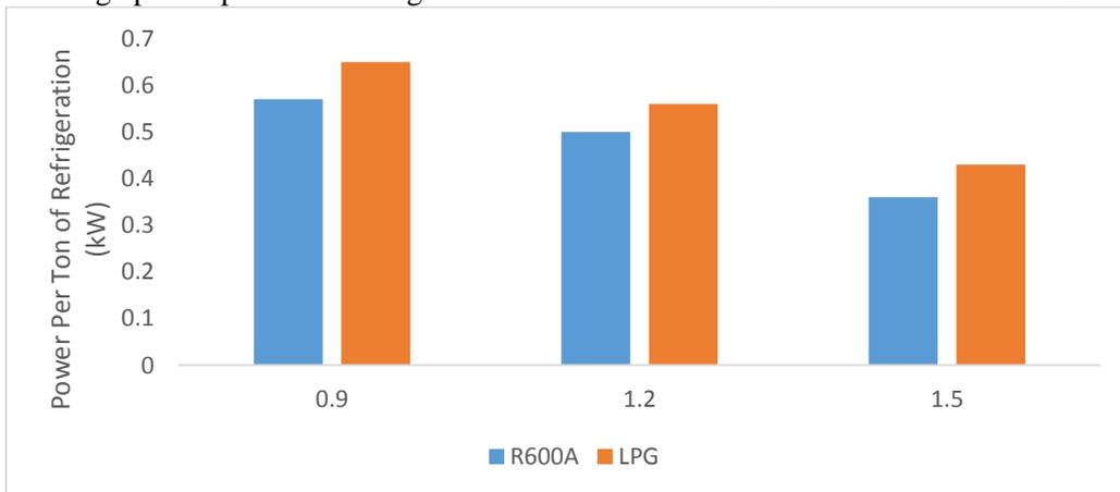
Figure 5: Effect of capillary tube on power per ton of refrigeration at Refrigerant Charge of 40g
