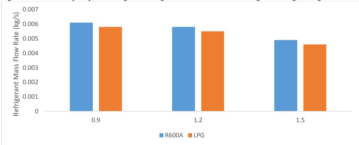
Figure 12: Effect of Capillary Tube Length on Refrigerant Mass Flow Rate at Refrigerant Charge of 40g
