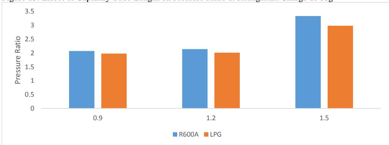
Figure 14: Effect of Capillary Tube Length on Pressure Ratio at Refrigerant Charge of 40g
