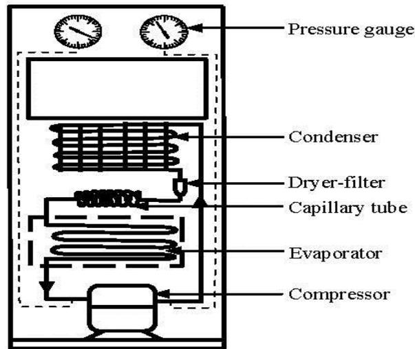
Figure 1. Schematic Diagram of Experimental Refrigerator.
