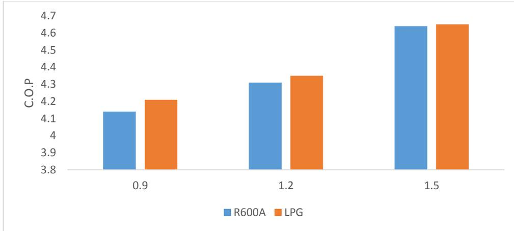
Figure 3: Effect of capillary tube length on the COP of the System at Refrigerant Charge of 40g.
