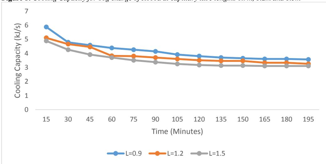
**Figure 9:** Cooling Capacity for 40g charge of LPG at capillary tube lengths 0.9m, 1.2m and 1.5m
