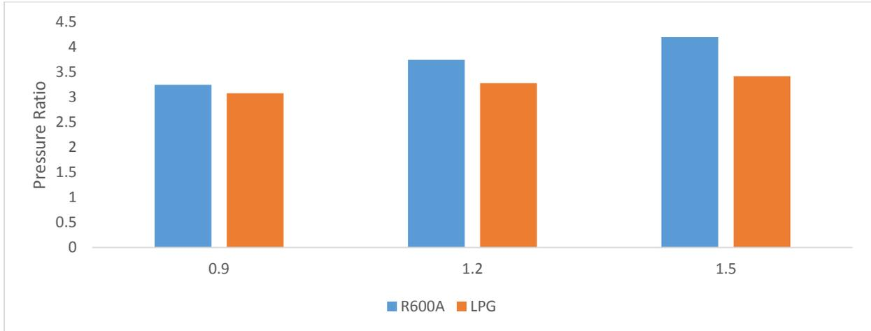
Figure 13: Effect of Capillary Tube Length on Pressure Ratio at Refrigerant Charge of 60g
