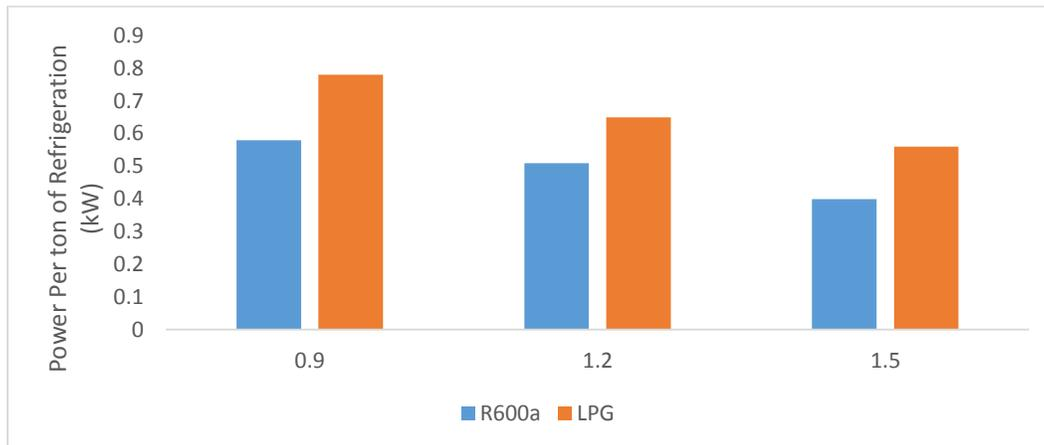
Figure 6: Effect of capillary tube on power per ton of refrigeration at Refrigerant Charge of 60g
