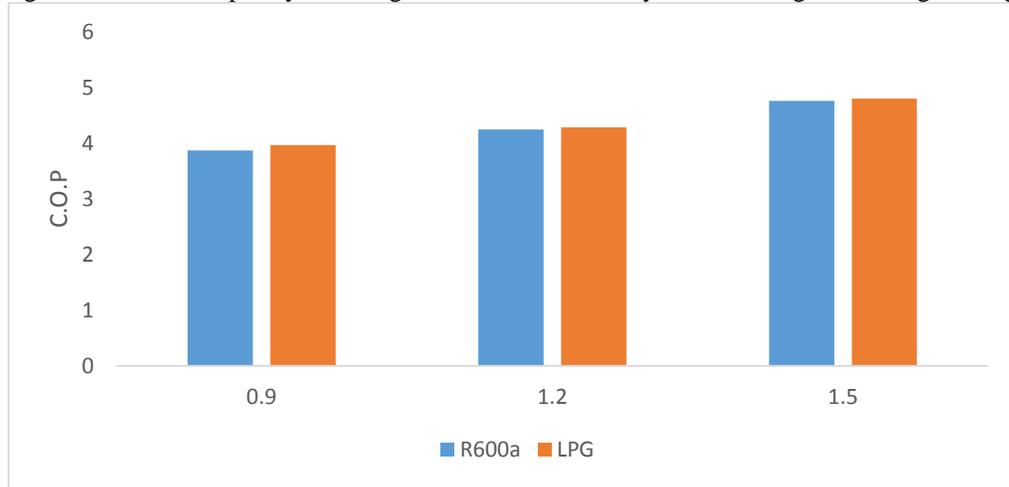
Figure 4: Effect of capillary tube length on the COP of the System at Refrigerant Charge of 60g.
