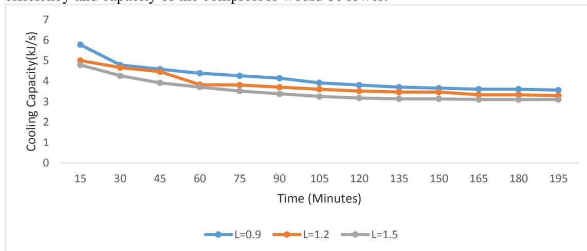
Figure 7: Cooling Capacity for 40g charge of R600a at capillary tube length 0.9m, 1.2m and 1.5m
