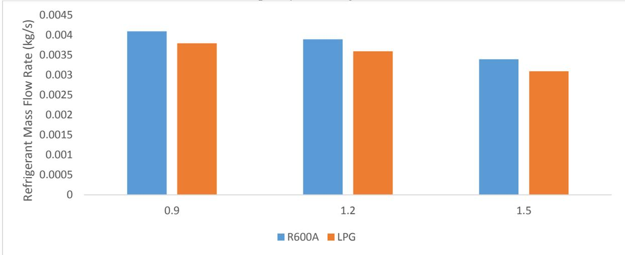
Figure 11: Effect of Capillary Tube Length on Refrigerant Mass Flow Rate at Refrigerant Charge of 60g
